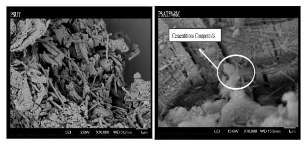
Fig. 2 FESEM images of natural (PSUT) and acid treated samples (PSAT5%8M).
