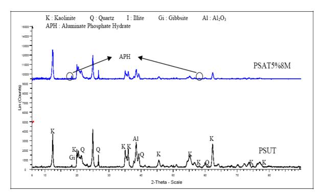
Fig. 1. XRD patterns of untreated (Bottom) and 5% phosphoric acid-treated soil (Top).
