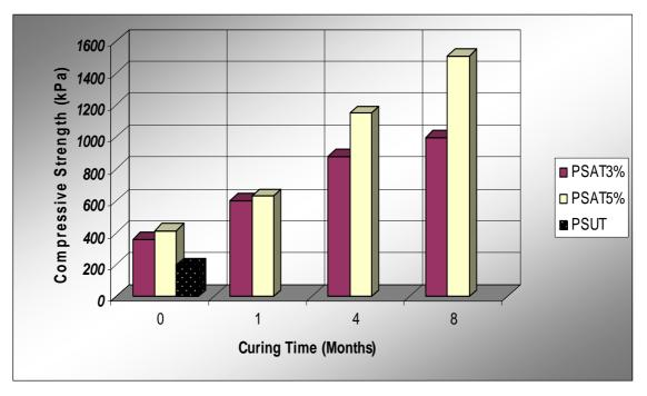
Fig. 3. Strength development for Pink Soil mix designs with curing time.
