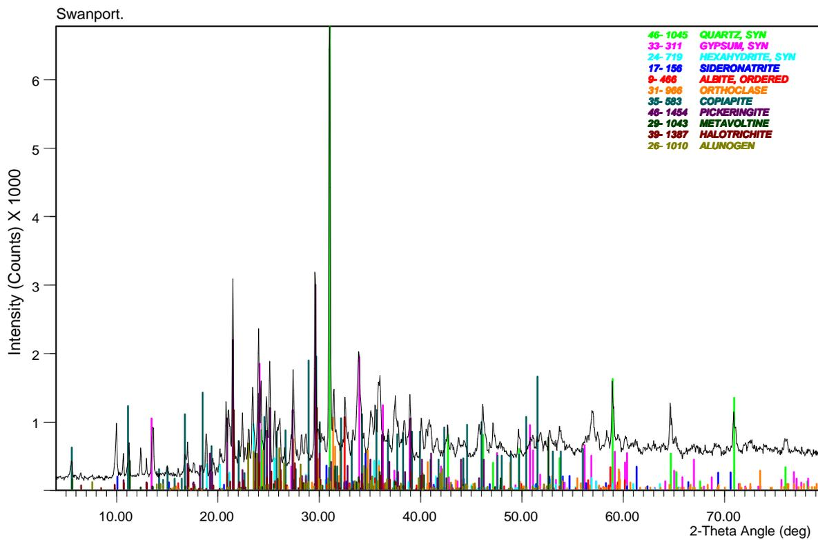
Fig. 2. XRD pattern (Co K $\alpha$  radiation) of sample collected from an ASS in the lower reaches of the River Murray (Swanport, SA).
