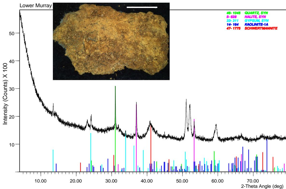
Fig. 3. XRD pattern (Co K $\alpha$  radiation) and image of a schwertmannite-rich sample collected from ASS in wetlands adjacent to the Finnis River, SA. Bar in image = 0.5mm.
