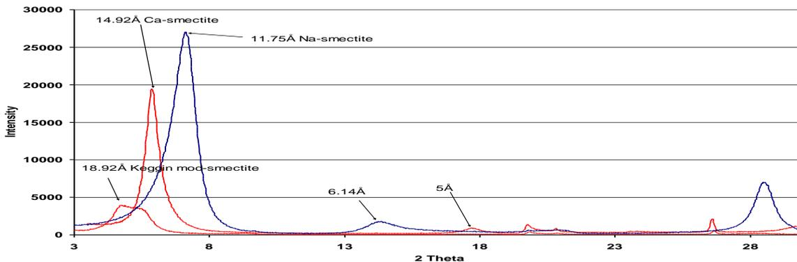
**Fig 1.** XRD pattern from Swy-2 montmorillonite sample modified using  $\text{Na}^+$ ,  $\text{Ca}^{2+}$  and Keggin  $\text{Al}_{13}^{7+}$  shown significant shift in the major peak from 001 distances between smectite layers.
