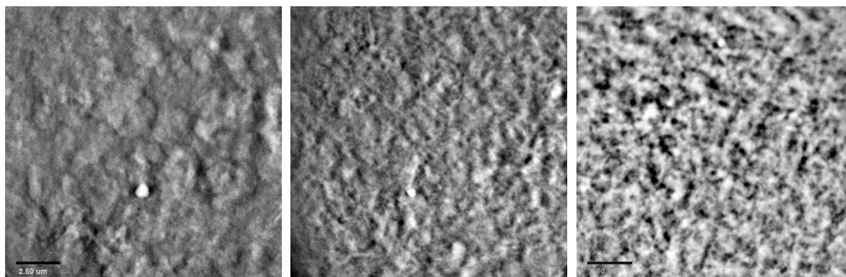
**Fig 2.** TXM micrographs of 5wt% (from left to right) Na, Ca, and  $\text{Al}_{13}$  treated montmorillonite colloidal gel in water; 2-D TXM micrographs. Scale bars are 2.5  $\mu\text{m}$ .
