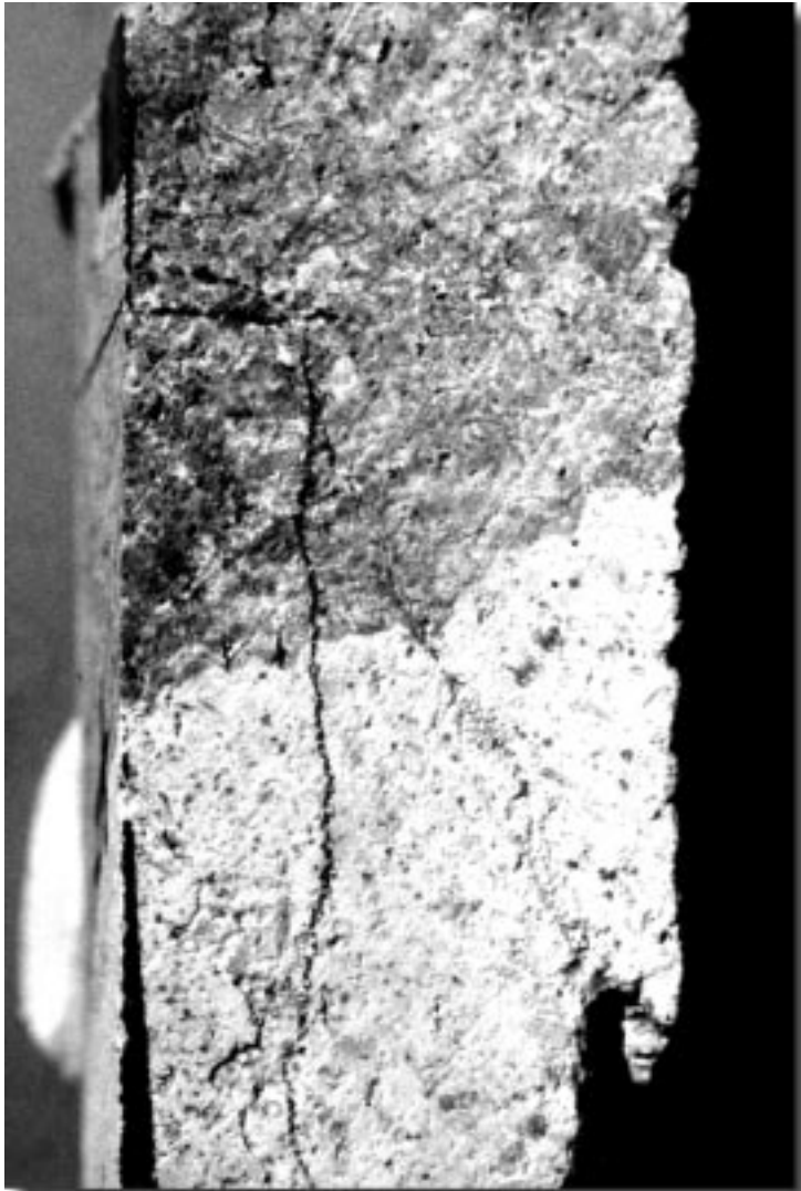
weathering front in a drill core marked by a change to darker colour. Keremenge, Papua New Guinea. (Photo I.D.M. Robertson)
