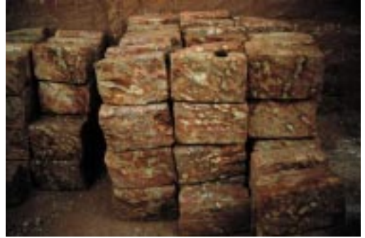
laterite bricks awaiting use, Angadipuram, Kerala, India. The material is vesicular mottled saprolite (Photo R.R. Anand)
