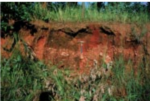
stone line profile showing red soil over quartz-rich stone line, Airforce-Mumba area, Zambia (Photo R. R. Anand)
