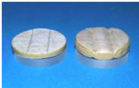
Figure 5. Hydrated stitch bonded GCL, showing the flat surface for a confined swell hydration (left), and the uneven surface for a free swell hydration (right)
